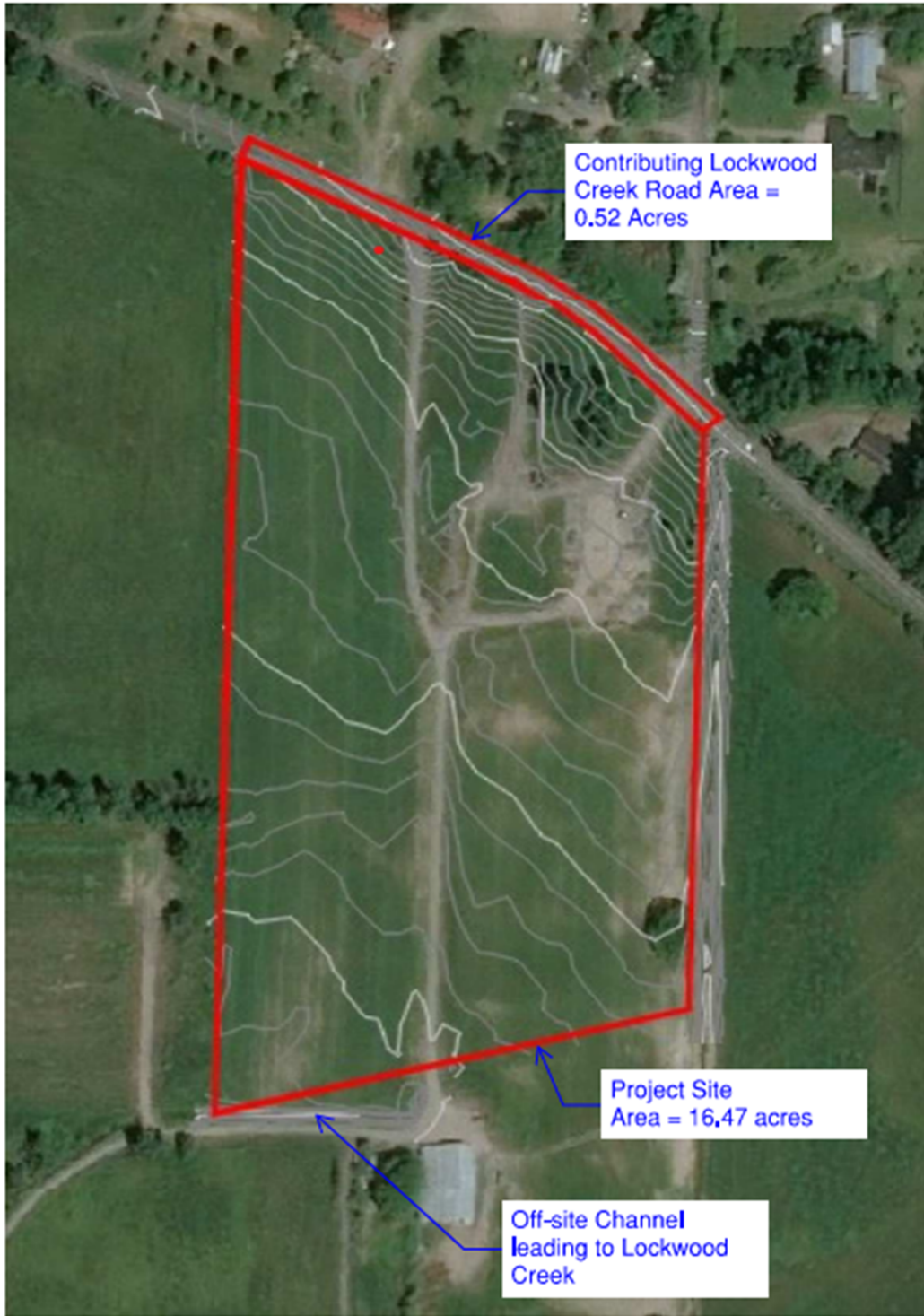
Figure 2. Existing Site Drainage Area
