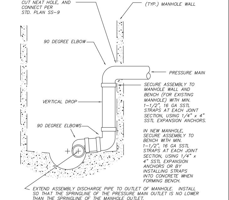
NOTE: PRESSURE MAIN CONNECTION ASSEMBLY MAY BE USED ONLY WHEN SPECIFICALLY APPROVED BY THE CITY ENGINEER.
