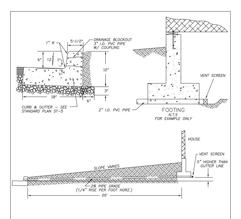
ALL LOTS MUST BE DESIGNED TO PROVIDE POSITIVE DRAINAGE FROM BOTTOM OF FOOTINGS TO AN APPROVED STORMWATER SYSTEM. POSITIVE DRAINAGE MAY BE ACCOMPLISHED BY SWALES, DRYWELLS, FRENCH DRAINS, LATERALS TO THE STREET, LATERALS BEHIND THE CURB OR WITHIN A PUBLIC UTILITY EASEMENT, AN APPROVED BACKYARD OR SIDE YARD SYSTEM, OR SOME OTHER METHOD ACCEPTABLE TO THE BUILDING OFFICIAL AND/OR DIRECTOR.
