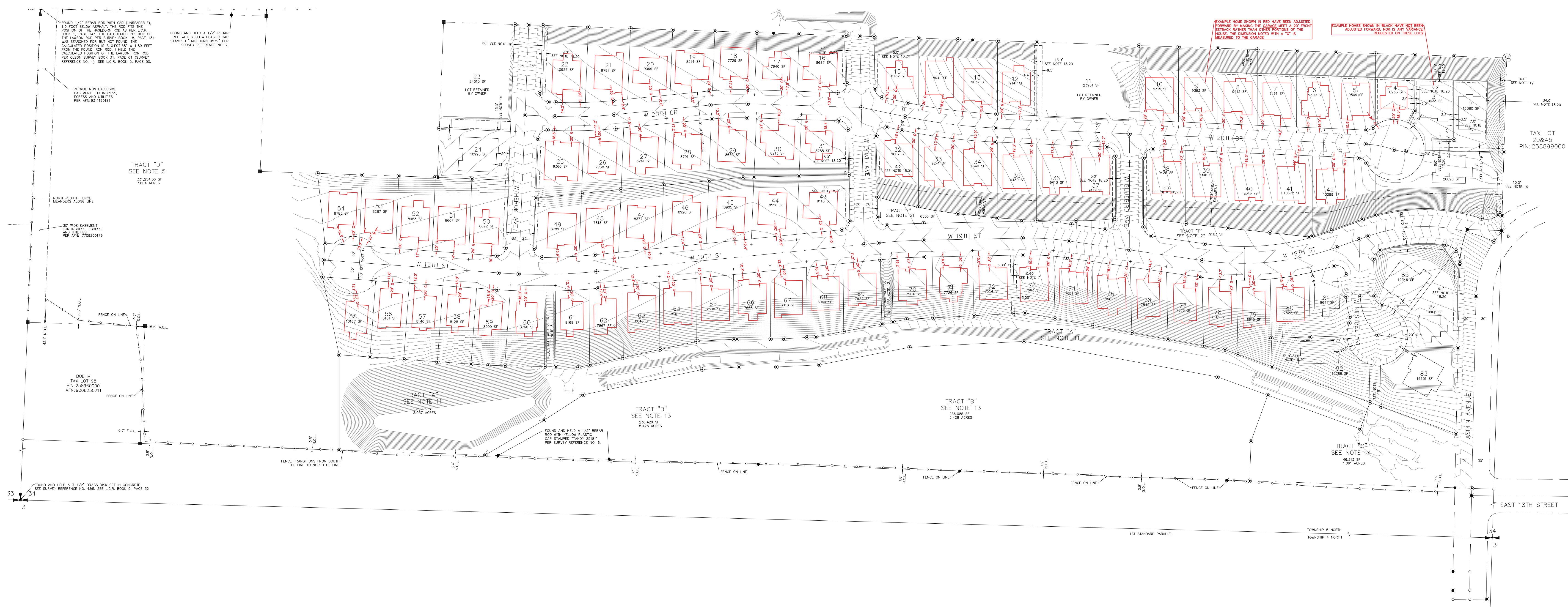
EXAMPLE HOUSE PLANS PLOTTED FOR "BEST USE" WITH VARIANCE TO FRONT BUILDING SETBACKS
