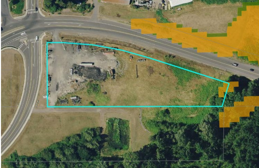
Figure 3: Areas of Potential Instability (in Orange)
