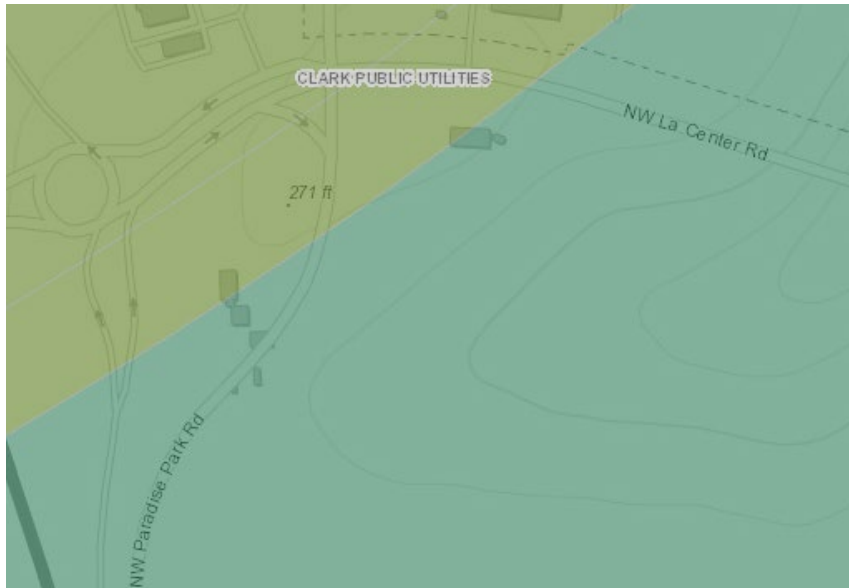
Figure 1: 5-year (Green) and 10-year (Blue) time of travel zone for Group A wellhead
