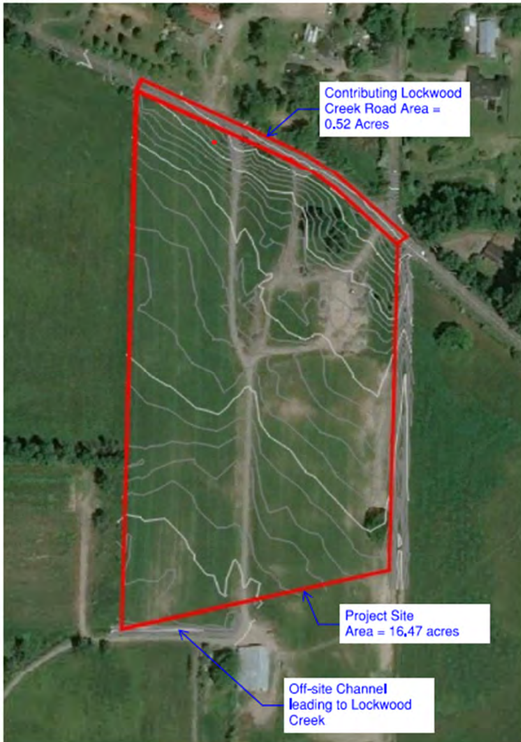
Figure 2. Existing Site Drainage Area
