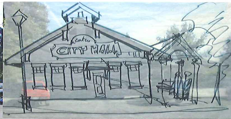
An Example of a Building Remodel to Meet Design Standards ~ A sketch analysis using the frontage of City Hall facing 4th Street as an example. This frontage currently has one solid door and no architectural detail. The sketch shows the addition of windows, a windowed door, awnings, craftsman style details on the roof face including a cupola, and a new covered entrance leading to the sidewalk. This type of renovation is relatively
